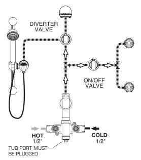
NOTE: MINIMUM FLOWING PRESSURE REQUIRED FOR THIS SYSTEM OPERATING WITH ONE SHOWER HEAD AND 2 BODY SPRAYS IS 40 PSI
